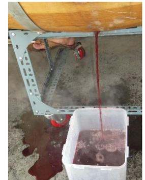
Steam Extraction of Tartrates from a Pre-cleaned Barrel
