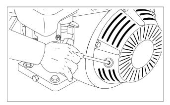
**STEP 9:** Pull the starter grip. If the engine fails to start after 2 pulls, squeeze the trigger gun to release pressure and repeat step. Return starter gently. After the engine warms up enough to run smoothly, move choke to run position and throttle to fast position.
