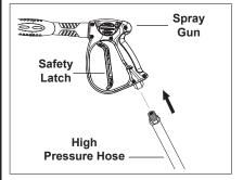
**STEP 4:** Attach the high pressure hose to the spray gun using teflon tape on hose threads.
