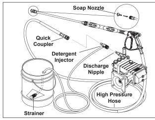
Connect high pressure hose to injector with quick coupler. (Check to make sure locking coupler sleeves are
