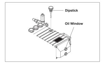
**STEP 2:** Remove shipping cap and install oil dipstick. Check pump oil level by using dipstick or observe oil level in oil window (if equipped). Use 30 wt. (non detergent) oil.
