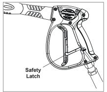
WARNING! Never replace nozzles without engaging the safety latch on the spray gun trigger.
