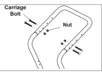
**STEP 2:** Insert the carriage bolt through the holes from the outside of the unit and attach a nut from the inside of the machine. Tighten nuts.
