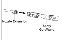
**STEP 5:** Attach nozzle extension to spray gun/wand. Tighten both by hand.
