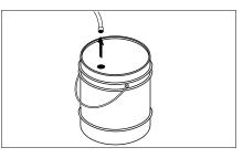
**STEP 1:** Remove detergent suction tube from container and insert into one gallon of fresh water. Slide nozzle forward for low pressure or to connect black detergent nozzle. Pull trigger on spray gun and siphon water for one minute.
