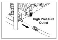
**STEP 6:** Disconnect the high pressure hose from high pressure outlet.
