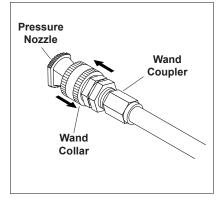
**STEP 3:** Release the coupler collar and push the nozzle until the collar clicks. Pull the nozzle to make sure it is seated properly.
