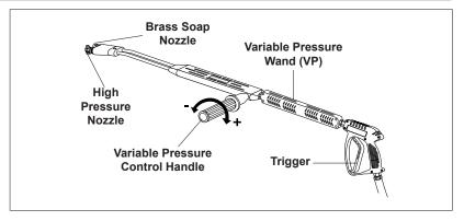
Selection of high or low pressure is accompanied by turning the handle. **Note:** High pressure nozzle must be inserted at end of wand to obtain high pressure. To apply soap read operator's manual.
